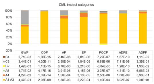
The production stage (module A1-A3) clearly dominates the LCA results. The loads caused by the disposal stage (modules C3 and C4) become noticeable especially in creating a major impact in the global warming potential (**GWP**). Transports play a subordinate yet not insignificant role.
